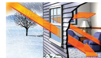
Winter Energy Savings: Low-E insulating glass reduces heat loss by reflecting warm air back into your home.
